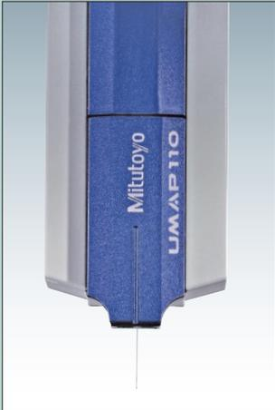
A stylus vibrating at an ultrasonic frequency enables the UMAP probe to sense contact with minute workpiece features. Five stylus tip diameters are available, from 15 to 300  $\mu\text{m}$ .
