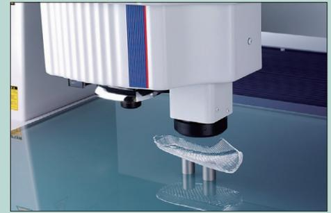
The Quick Vision Hybrid Type 4 is a machine which allows vision measurement with a CCD camera and high-speed scanning with a non-contact displacement sensor.
