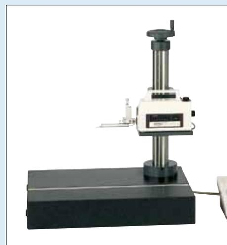
The SJ-500 can also be mounted on a manual column stand.
